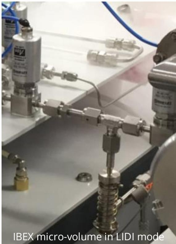
Once the sample has been cleaned, it is passed to the IBEX micro-volume for cryo-focusing and transferred to the mass spectrometer for analysis.
