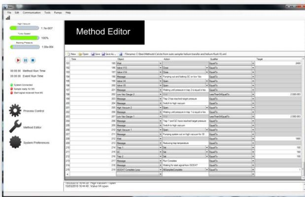
Custom analytical methods can be created using the ICC method editor. This requires no prior scripting or coding knowledge. New methods can be created and deployed in minutes.
