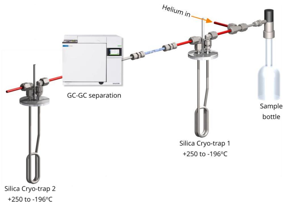
The cryo-traps use a variable head-pressure system to raise and lower the liquid nitrogen level without physically moving the trap. This provides safe and accurate trap cooling and heating.
