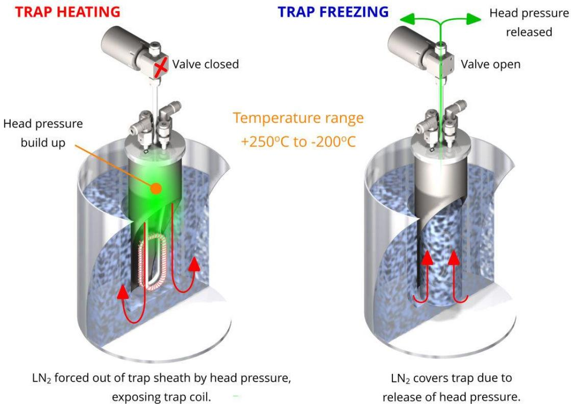
As the freezing point of CH<sub>4</sub> is close to LN<sub>2</sub> temperatures, a silica stationary phase is added to the IBEX cryo traps. This ensures near 100% recovery of CH<sub>4</sub> samples.
