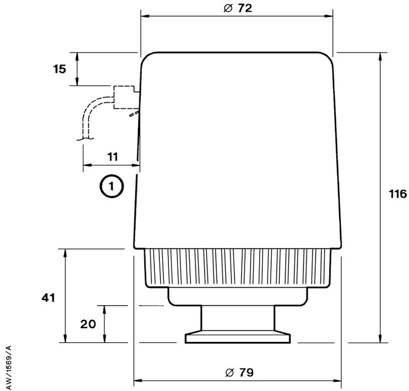
1. Clearance required for electrical cable
